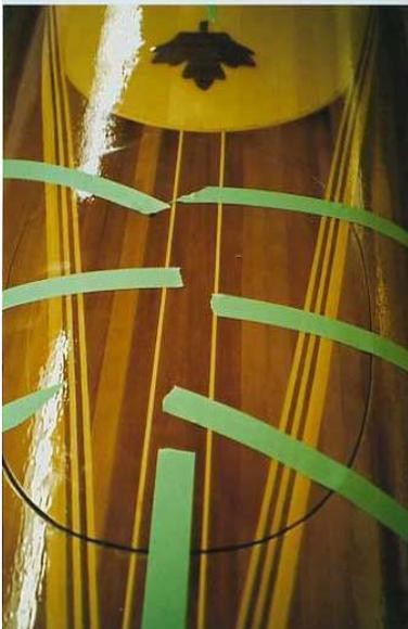
Cut the hatch openings  $\frac{1}{2}$  inch larger than the pattern provided (total extra diameter size – one inch). When cutting the scrap pieces for your hatch lips, make the pieces at least  $\frac{1}{2}$  inch longer than explained in the standard instructions. Extend this extra length into the hatch opening when gluing to the underside of your deck.
